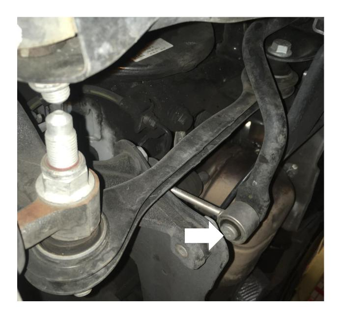
**Step 6:** Remove the bolts from the sway bar brackets for sway bar removal. T50 inverted Torx bit is required for removal.
