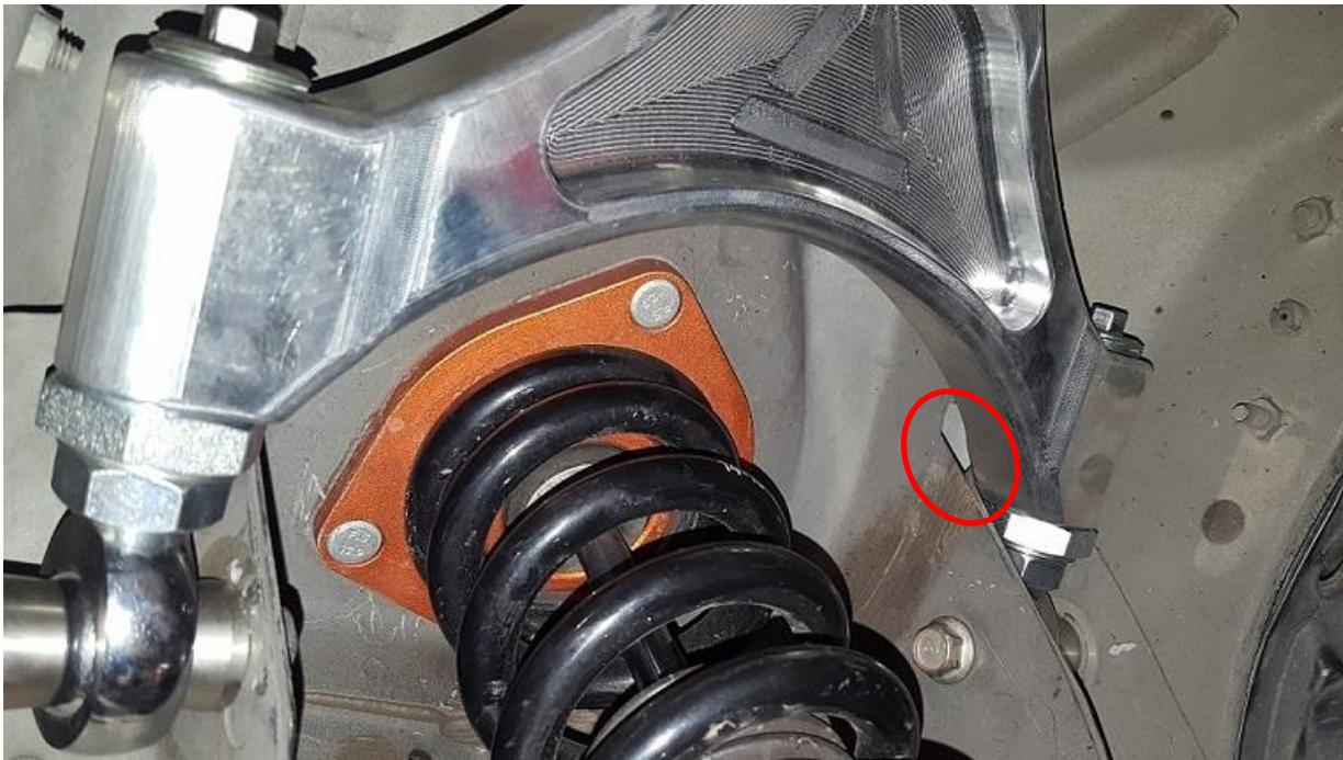
**Step 4:** Lifting the upper control arm out of the way, bring back the set aside upright and insert the ball joint shank into the appropriate mounting hole on top of the spindle. Reinstall factory cross bolt and nut and torque to 43 ft-lbs.
